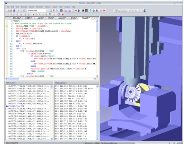
*Integrated APT/CL, G-code and machine view provide the complete picture for CNC post development.*
